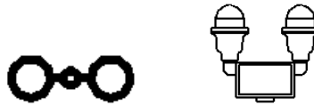
Figure 11: Left: Plan view of the obstruction double. Right: Elevation view of the fixture.
