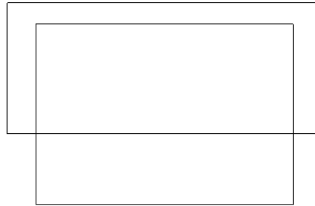
Figure 2: Plan view of a three phase, pad mount, transformer. The core and coil are in the main box, while the radiator for cooling is the attached box.
