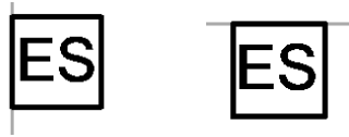
Figure 5: Plan view of the double door, electric strike (ES): Left – sideways, Right – upright.
