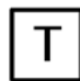
Figure 17: Plan view of the pad mounted, indoor transformer. The transformer family only shows the symbol, not the actual dimensions. This is intended only for small indoor transformers, where the dimensions are too small and so a symbol is used.
