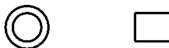
Figure 3: Plan view of the underground circular hand hole. The rectangular version is shown on the right and circular version shown on the left.
