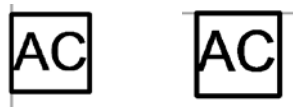
Figure 12: Plan view of the access control door status magnetic switch (AC): Left – sideways, Right – upright.
