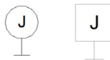
Figure 12: Plan view of the vertical mounted junction box. Left – small J-box symbol, Right – large J-box symbol
