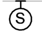
Figure 4: Plan view of the speaker, wall mounted. The 3d view of this speaker is recessed into the wall.
