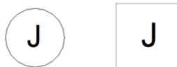
Figure 10: Plan view of the ceiling mounted junction box. Left – small J-box symbol, Right – large J-box symbol
