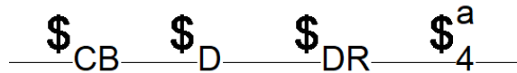
Figure 1: Plan view of the sample switches. The subscript indicates the switch type (circuit breaker, dimmer, door, 4-way, double pole, single pole, etc) and the superscript indicates the switch ID or the controlling circuit. The controlling circuit indicates which lights the switch will control. See the built in types in the table below for a list of available switch types.
