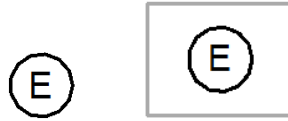
Figure 29: Plan view of the electrified equipment symbol. Non-hosted on left and hosted on right.
