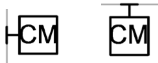
Figure 8: Plan view of the access master unit (CM): Left – sideways, Right – upright.
