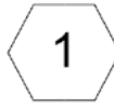
Figure 4: Plan view of the hexagon keynote. This does not use the built-in keynotes for Revit®.
