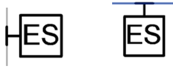
Figure 9: Plan view of the single door, electric strike (ES): Left – sideways, Right – upright.
