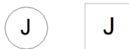
Figure 11: Plan view of the ceiling mounted junction box. Left – small J-box symbol, Right – large J-box symbol
