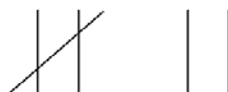
Figure 4: Normally closed and normally open contact, one-line diagram symbols on drafting view (1:1 scale).
