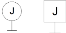
Figure 8: Plan view of the wall mounted junction box. Left – small J-box symbol, Right – large J-box symbol
