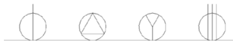
Figure 1: Plan view of the wall mounted, single receptacles. From left to right – Special Purpose 120V, Special Purpose 240V, Special Purpose Three Phase, and Range.
