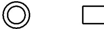
Figure 4: Plan view of the underground rectangular hand hole. The rectangular version is shown on the right and circular version shown on the left.
