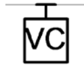
Figure 6: Plan view of the volume control station, wall mounted. The 3d view of this station is NOT recessed into the wall; it is placed on the surface.
